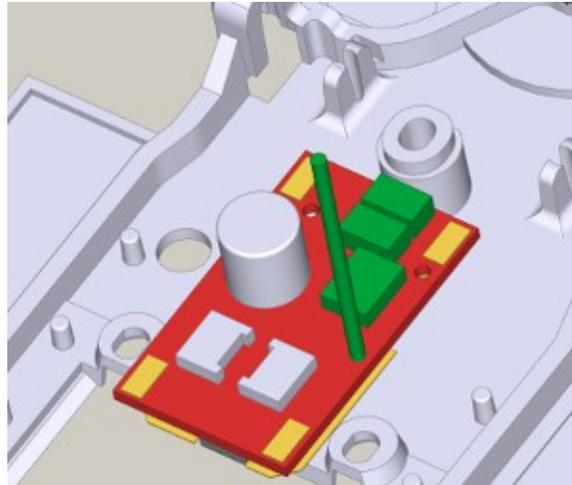
Once the chip is properly placed inside the car chassis, make sure the LED can be seen through the chassis hole. The chip also provides extra pads to wire an external additional lane changer LED. There is no need to remove the standard LEDs, which are mounted directly on the board. If you are running on Carrera D132 instead of oXigen or SSD, use the wired LED and place it so that it aligns with the Carrera receiver that can be found on the track, right before the lane changing mechanism.
