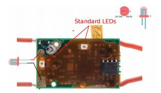
A "kapton" protective cover is glued to the bottom side of the chip to protect the electronic components. Don't remove this protection to avoid damaging the chip and loss of warranty.
