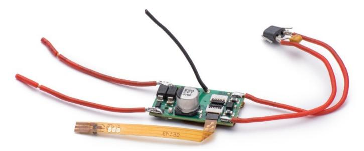
It's a universal unit, being natively compatible with oXigen, Scalextric SSD, and Carrera digital. 'Compatible' means that the chip performs like any SSD or Carrera 132 original system once the proper software is loaded. In other words, when appropriately programmed, you can use this chip on either Scalextric SSD, or Carrera D132, as if it was a 'standard' device for the said system.
