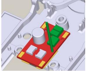
Once the chip is properly placed inside the car chassis, make sure the LED can be seen through the chassis hole. The chip also provides extra pads to wire an external additional lane changer LED. There is no need to remove the standard LEDs, which are mounted directly on the board. If you are running on Carrera D132 instead of oXigen or SSD, use the wired LED and place it so that it aligns with the Carrera receiver that can be found on the track, right before the lane changing mechanism.
